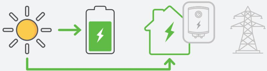
Automatic diversion of solar energy to priority loads when batteries are full, avoiding export
